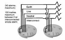
WARNING: Connection to the EARTH terminal is not needed for correct functioning of the Smoke Alarm. It is just for conveniently terminating any earth supply wire coloured green or green/yellow. It does not provide protective earthing for the Smoke Alarm
