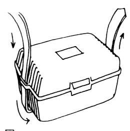
Pass the strap DOWN through the first case lug, under the case and UP through the other lug.
